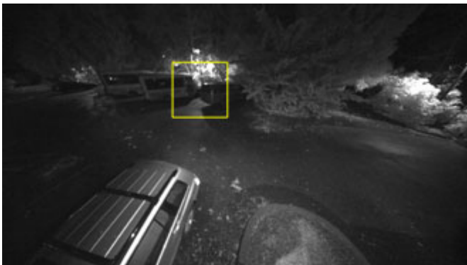
Under the same conditions except replacing the standard lens with a day/night lens such as Theia's new SY110 lens keeps the image in focus day and night.
